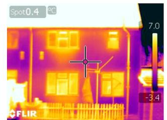
Thermal image of the building prior to work commencement, bright colours indicate high heat losses from central heating radiators
